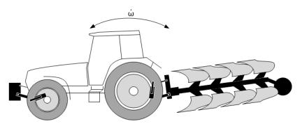
Figure 1: Pitching movement of an agricultural tractor with front weight and plough.
